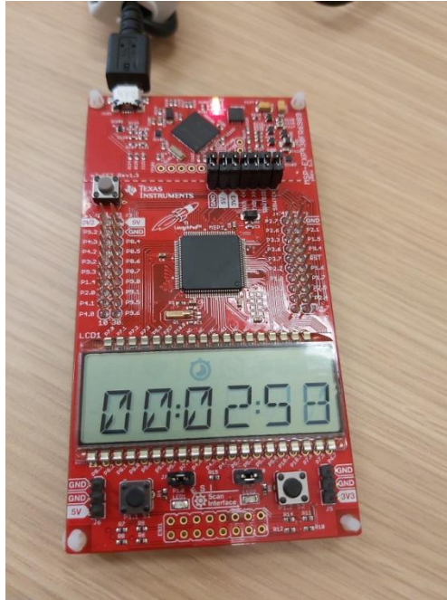
Fig. 3.1. Stopwatch on TI MSP-EXP430FR6989.
