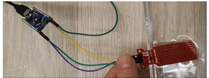
Fig. 2.2. Assembled prototype for water sensor with Arduino Nano Every. The water sensor is submerged into water.
