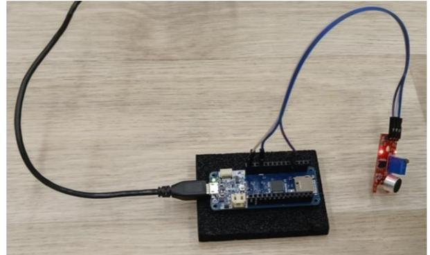
Fig. 4.2. Assembled sound sensor with Arduino MKR Zero.
